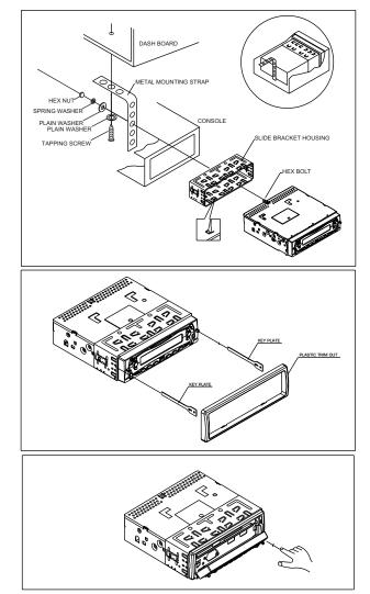
If you want to take CHASSIS out of the SLIDE BRACKET HOUSING, remove the PLASTIC OUTLINE away, then insert the two KEY PLATE into left and right side of chassis as above illustration.
